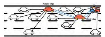
Fig. 4. Edge-based multi-hop broadcast.
