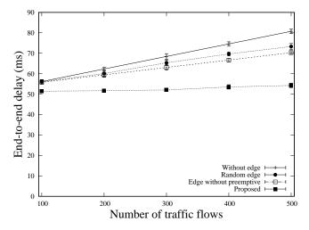
Fig. 8. End-to-end delay for various vehicle densities.
