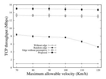
Fig. 6. TCP throughput for various vehicle velocities.
