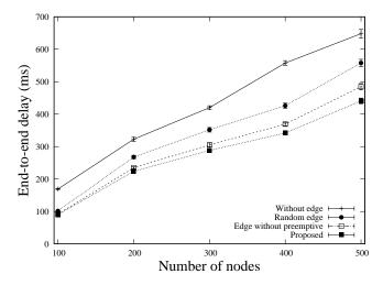
Fig. 12. End-to-end delay for various vehicle densities.
