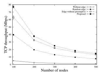
Fig. 5. TCP throughput for various numbers of receivers.
