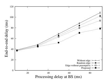
Fig. 9. End-to-end delay for various processing latencies at the base station.
