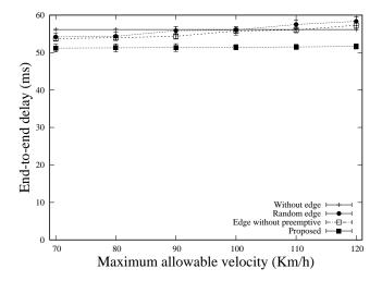
Fig. 10. End-to-end delay for various vehicle velocities.
